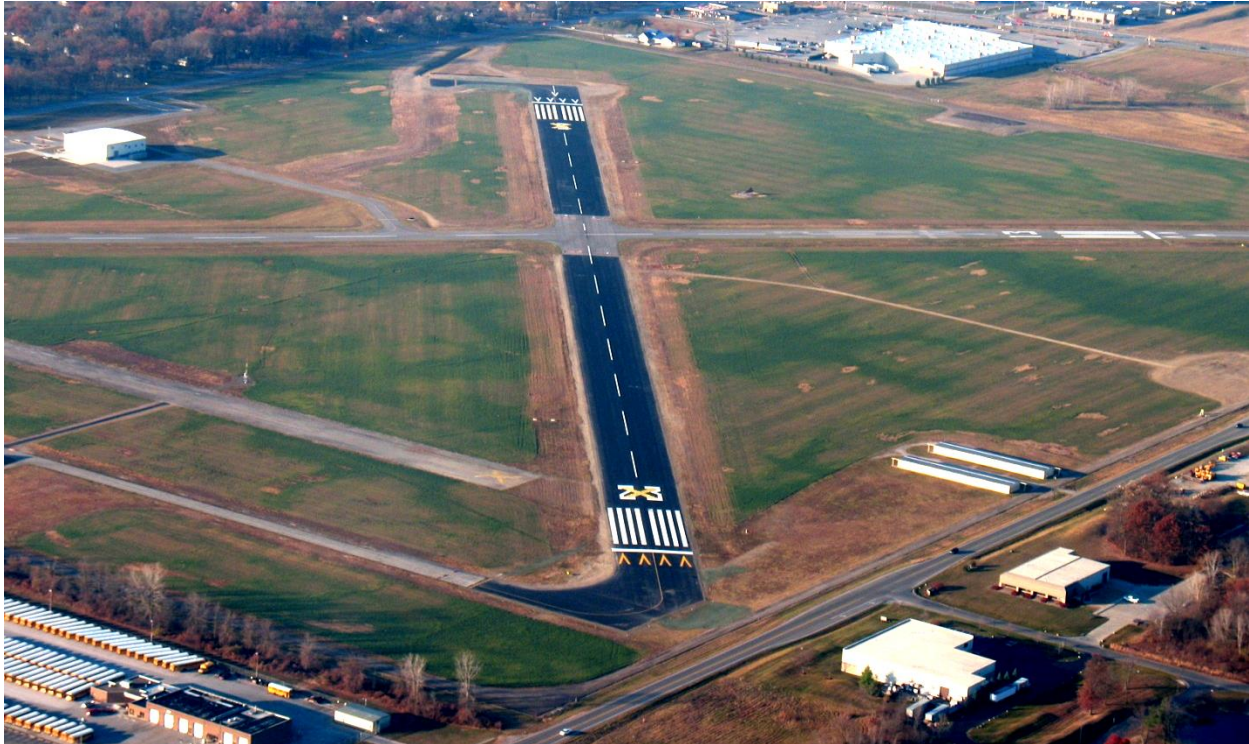
Figure 2-3. Markings for a Temporarily Closed Runway
